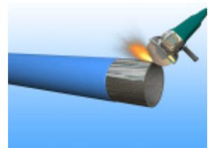
7. Before butt welding water line pipes, cut back the cement mortar lining 3-5 mm at the pipe ends using a special angle grinder attachment (see list of accessories).
