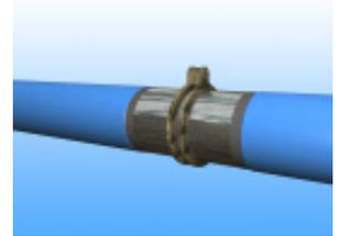
4. Depending on the welding conditions and the pipe material used, the pipe ends may have to be preheated as specified in the welding instructions.
