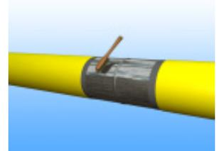
2. Apply primer in accordance with the manufacturer's instructions. It may be necessary to let the surface dry before applying the primer. Observe flash-off time requirements before wrapping the anticorrosion tape round the pipe joint.
