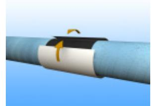
2. Use the supplied adhesive tape to fix the mould in the centre of the filling slot. This ensures a uniform annular space around the pipe. Secure the mould in position with adhesive tape. Pull firmly, lapping the tape around the circumference at both ends of the mould to seal it off.
